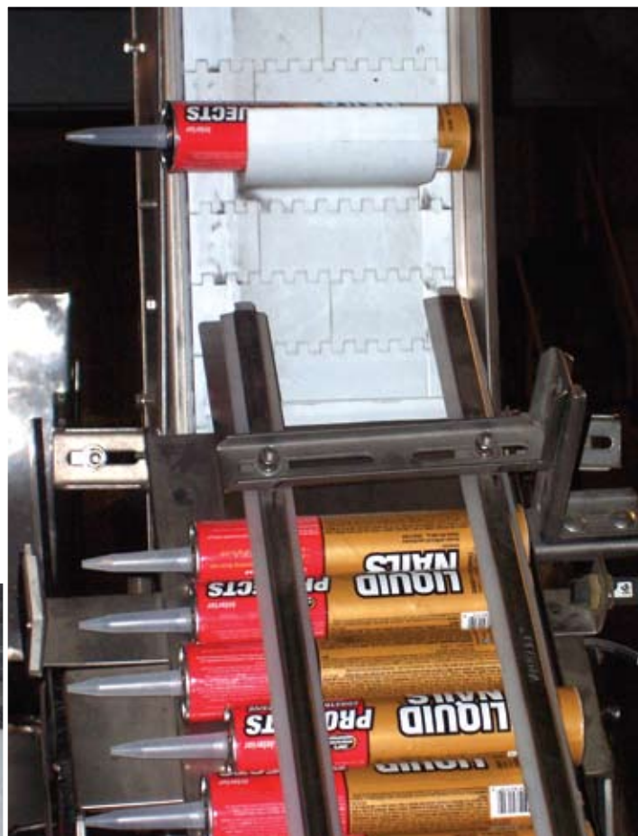
STAR WHEEL. A flighted takeaway conveyor (above) carries individual cartridges from the overhead orienting bowl down to a chute that feeds cartridges into a servo-driven star wheel (left).
