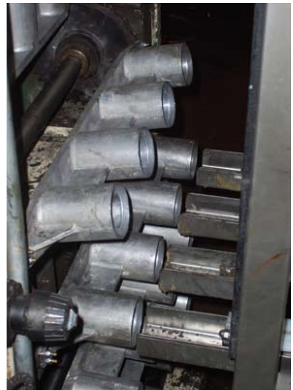
FILLER INFEEED. The new infeed system places empty cartridges in these pockets on the four-lane volumetric filler.
