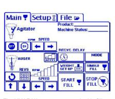
The NMAF-X2 sets a new standard in filling technology with a computer controlled digital servo motor drive and operator touch screen interface. The computer controlled brushless direct drive servo motor system provides superior fill accuracy and reliability. The user friendly graphic menu allows the operator to easily access product memory for fast set-up and accurate control of filling operations.
